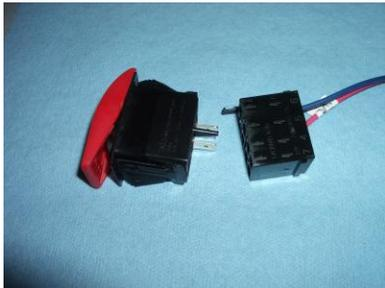
Now grab the wiring loom that came with your Horn kit. The plug at the end of the wires will push onto the back of the toggle switch. From behind the panel that you installed the switch into, hold the plug so that the locking tab is aligned properly with the small square hole on the back of the switch body. Push onto the back of the toggle switch.
